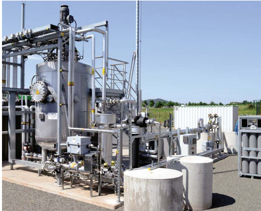
World's first power-to-gas plant with biological methanation in Allendorf (Eder)
