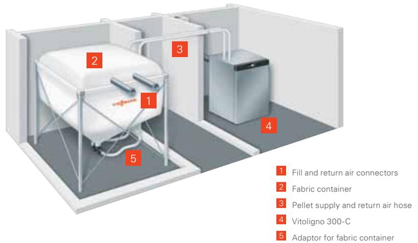
Storage room without sloping floor with supply to the pellet boiler via suction wands
