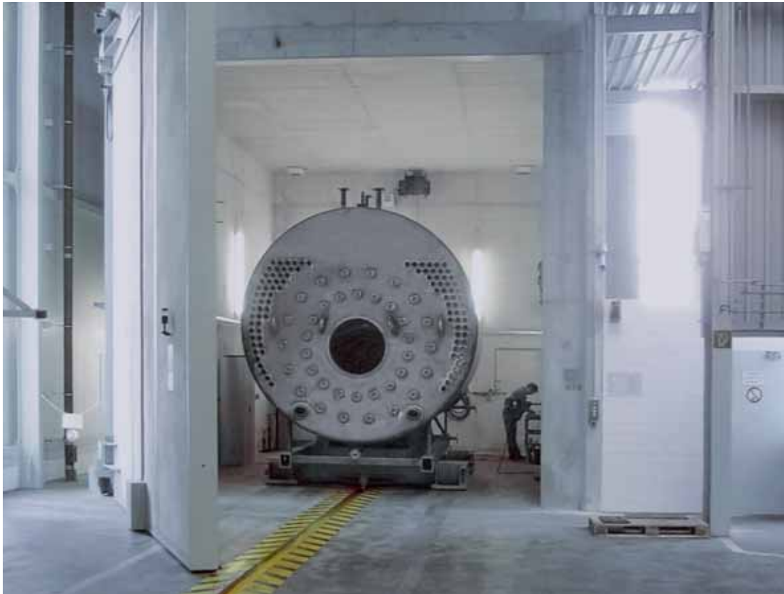
Boiler assemblies and entire Vitomax boilers are inspected for fault-free weld seams and material weakness inside the X-ray chamber.
